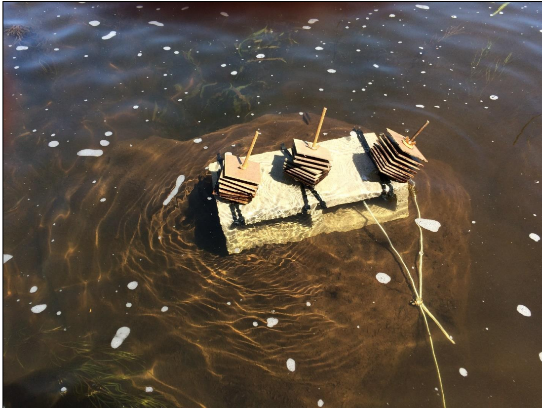
Figure 6. Photograph of H-D samplers attached directly to a cinder block prior to deployment at a shallow (<1.5 m), firm bottomed site.
