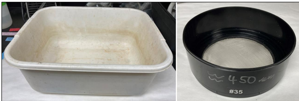
Figure 9. A dish pan ( left ) is ideal for holding H-D samplers immediately after removing them from the water so invertebrates do not escape. Any light-colored pan will work for this purpose. A sieve can be used as well. Any screen or mesh should be between 400 and 500 \mu m.
