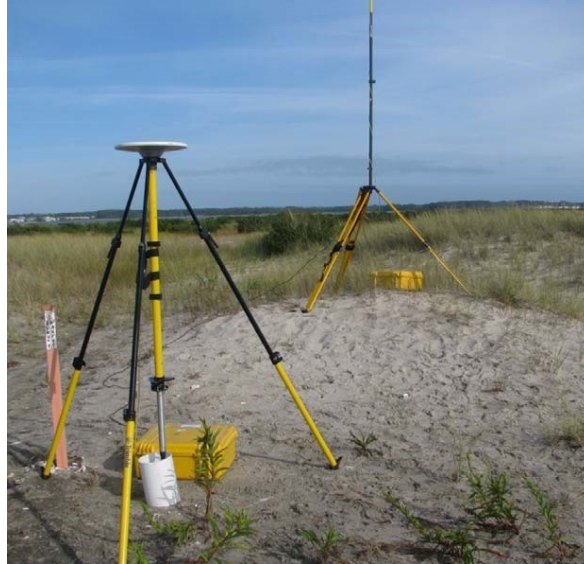
Figure S2.2. The Trimble 5700 Base station setup: in the foreground, the Zephyr geodetic antenna and the base receiver (inside the case), and in the background, the radio transmitter antenna (TRIMMARK 3 from Trimble) (Assateague Island, September 2009).
