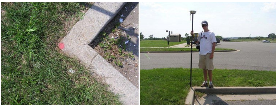
Figure S3.4. Monument location at corner of curb of a traffic island on a parking lot at Great Kills, Gateway National Recreation Area; adequate space for a GPS/GNSS base station or rover receiver pole (Staten Island, New York, August 2008).
