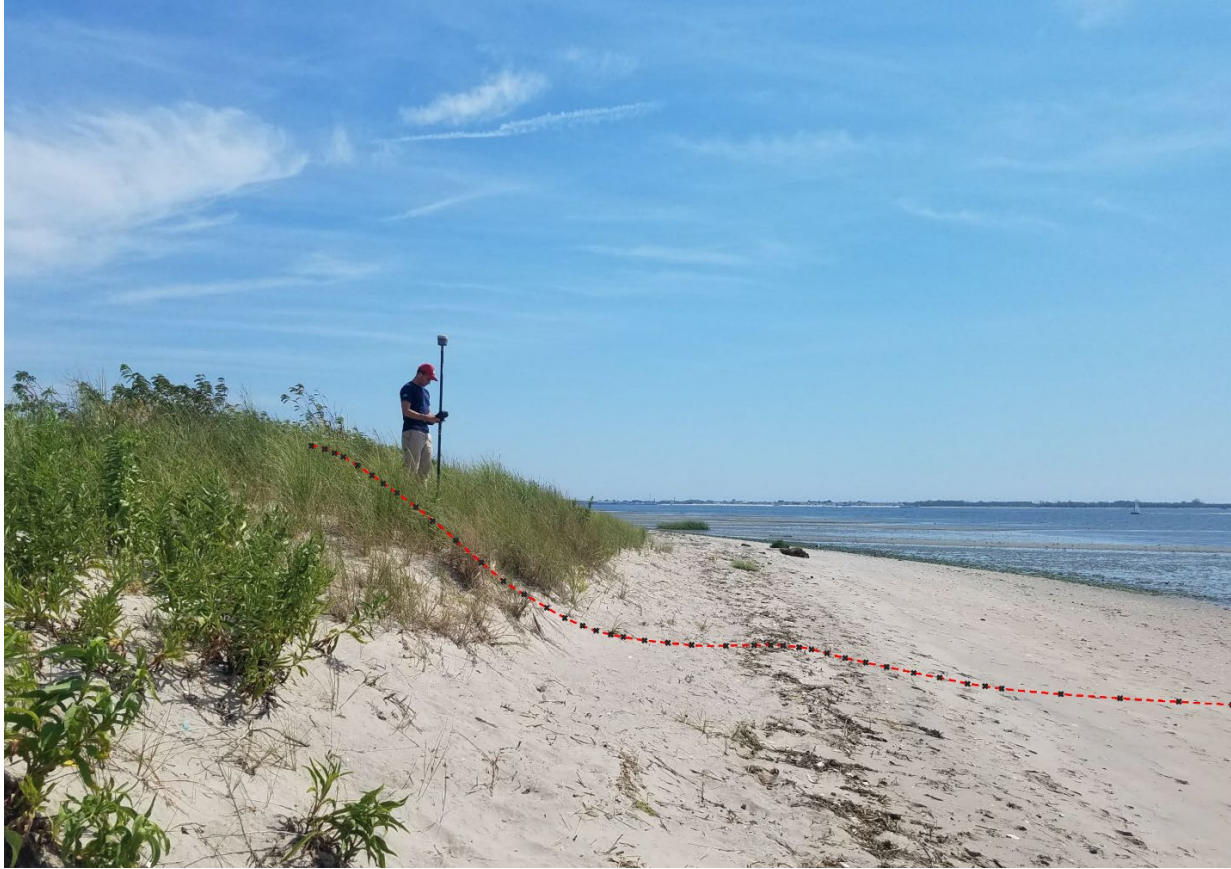
Figure S7.6. Measurement of topographic points along a transect at Plumb Beach, within the Jamaica Bay Unit of Gateway National Recreation Area. Example of points being measured at change in slope: at top and bottom of the feature.
