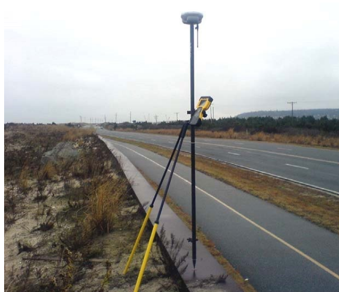
Figure S2.1. The Trimble R8 GNSS receiver and Trimble TSC2 field survey controller (Sandy Hook, New Jersey, November 2009).
