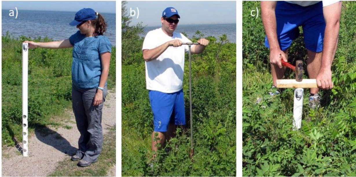
Figure S3.5. PVC pipe monument; a) PVC pipe with holes; b) coring in field, and c) final driving of PVC pipe into sand.
