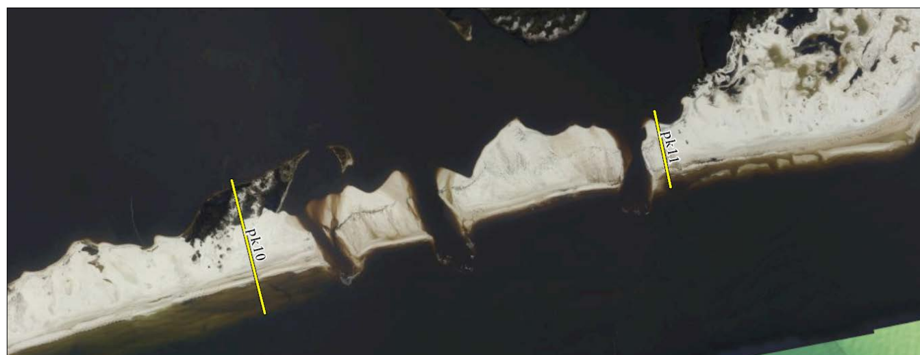
Figure 7. Image courtesy of NOAA Remote Sensing Division, taken soon after Hurricane Sally in September 2021, shows breaching in the overwash zones between transects PK 10 and PK 11.
