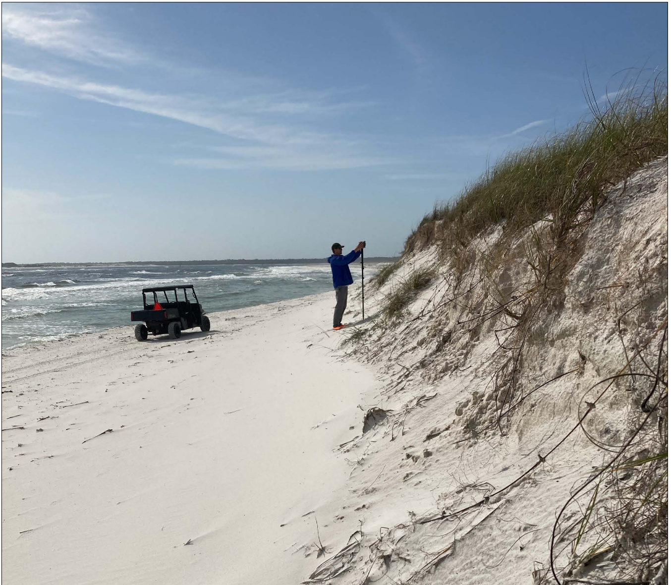
Figure 2. Surveyor measuring beach/dune topography taken in April 2021 at Fort Pickens, Gulf Islands National Seashore. NPS photo / GULN staff.
