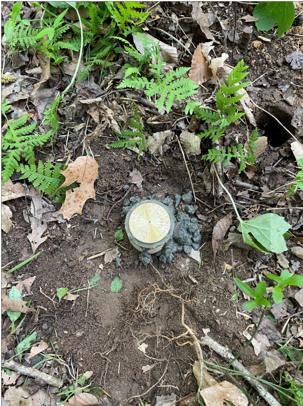
Figure 4. Example of a secondary benchmark (BM1S) placed on each detailed cross-section during the initial site assessment.
