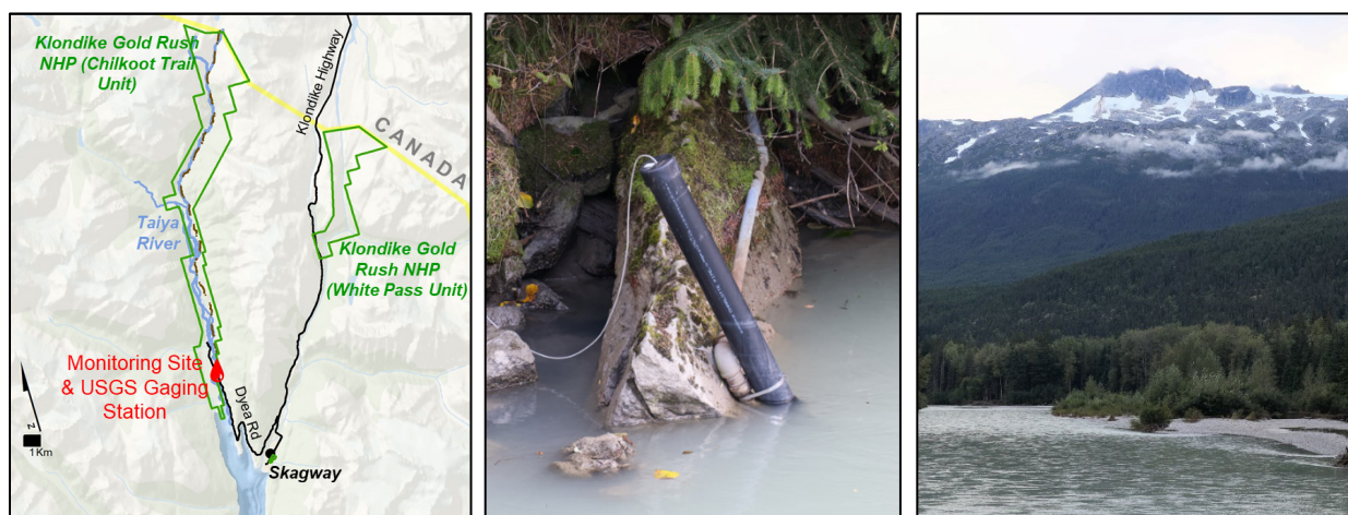
Figure 3. SEAN monitoring site and co-located USGS gaging station on the Taiya River at KLGO. Location map (left), sonde (center), and immediate downstream reach (right).
