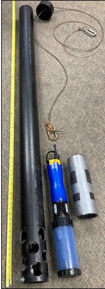
Figure 5. Example of sonde housing and installation accessories from the Taiya River. Housing cap, foam (with duct tape reinforcing shape), and tether shown alongside plastic pipe housing and EXO3 multiparameter sonde with calibration cup.
