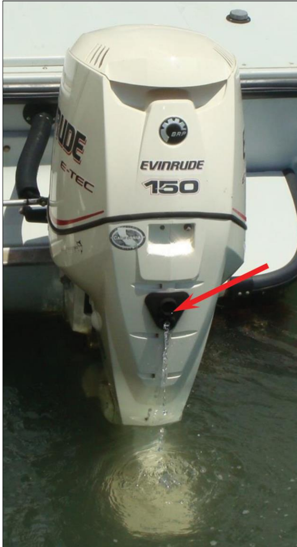
Figure A-3. Water pump indicator.
