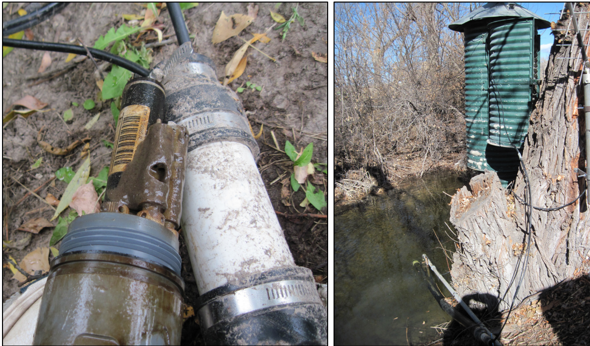
Figure 3. A sonde device is used to measure water quality in the Niobrara River at Agate Fossil Beds National Monument. The United States Geological Survey Niobrara River gaging station (06454100) is set up for real-time data transmission via satellite. Photographs courtesy of KA McLaughlin, RE Woodruff & KRW, of the USGS, at Station 06454100.
