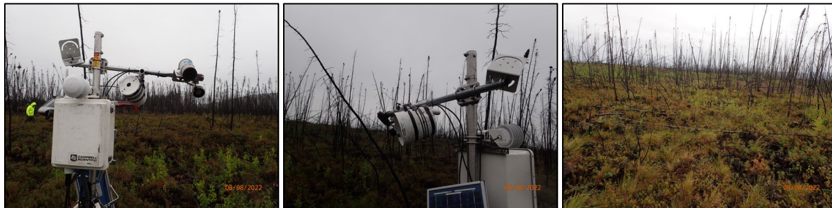
Figure 13. Andrew Creek Fire station on August 8, 2022, with damage from bear (left, middle) and after station was removed (right).
