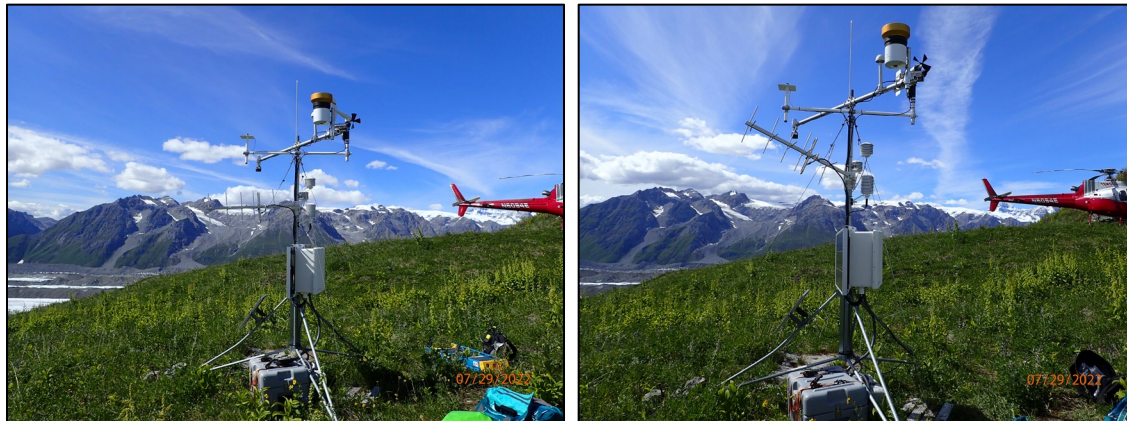
Figure 8. Gates Glacier climate station, July 29, 2022. Antenna out of level on arrival (left) and station at end of site visit (right).
