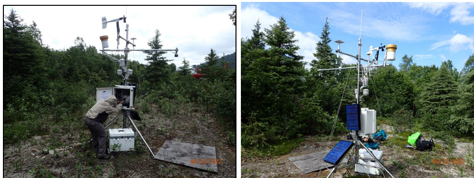
Figure 3. Stampede climate station, June 23, 2022. The tipping bucket was out of level on arrival (left) end of site visit photo (right).
