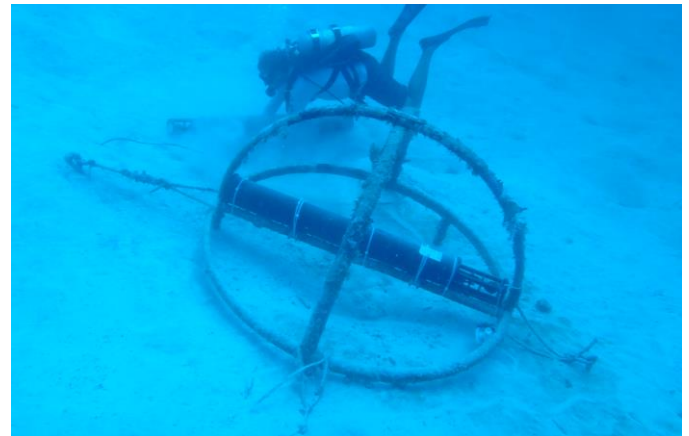
Figure 3: Bioacoustic monitoring site near BUIS. The hydrophone recording package (NOAA PMEL) was attached to a protective metal lander and secured to the seafloor with sand screws. The hydrophone package is swapped annually for data download and re-programming by NPS dive staff. Photo: National Park Service
