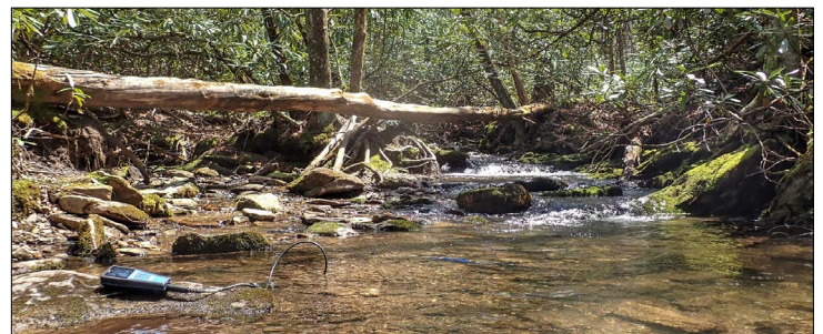
Multi-sensor sonde measuring water quality in a stream. NPS photo / APHN staff.
