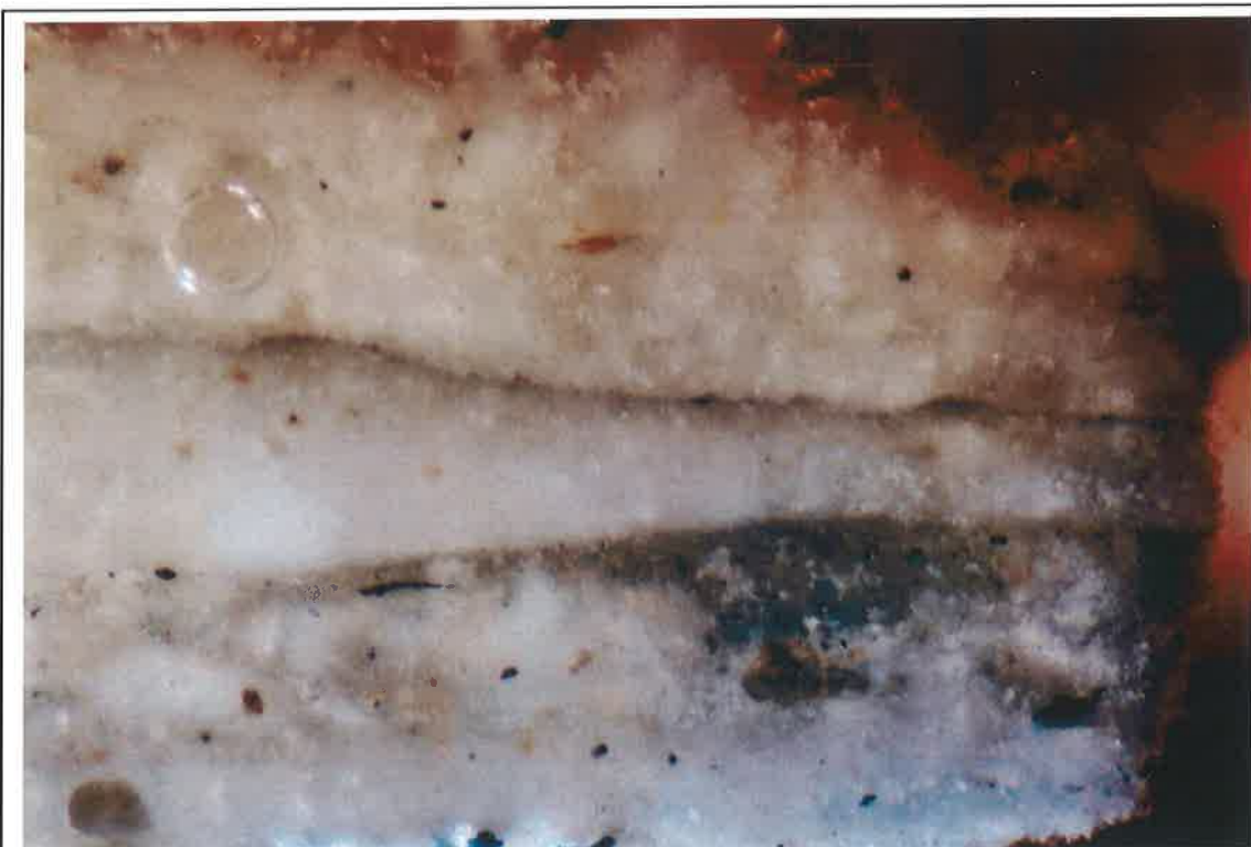
Image 83: Oakland Plantation. South Tenant Cabin, west elevation. Photomicrograph of the three layers of limewash found on a fragment of Door D5. (Sample #OPST.57, 10x mag.).
