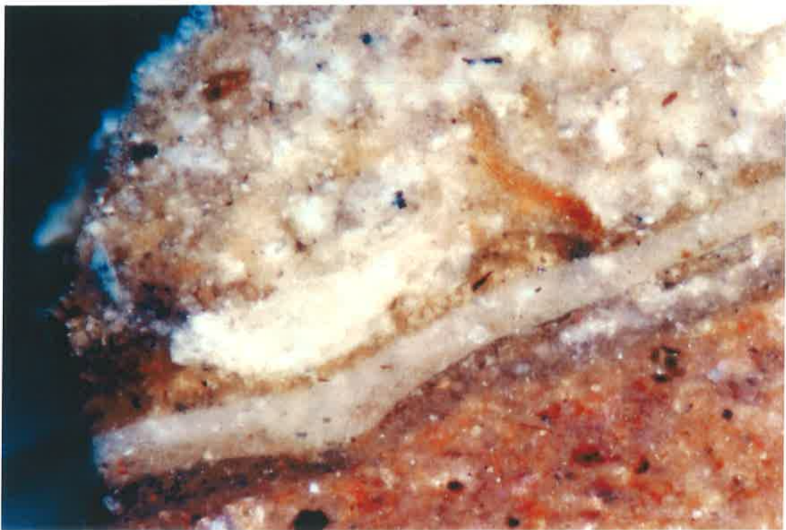
Image 73: Oakland Plantation. South Tenant Cabin, Room 102, 2002. Photomicrograph of Sample #OPST.14 (10x mag.) showing the whitewash layers on the bousillage of the north wall.
