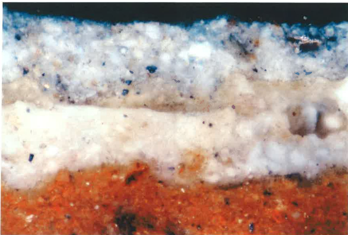
Image 69: Oakland Plantation. South Tenant Cabin, 2002. Photomicrograph of Sample #OPST.1 (10x mag.) showing the layers of limewash on the original bousillage on the east wall of Room 104.
