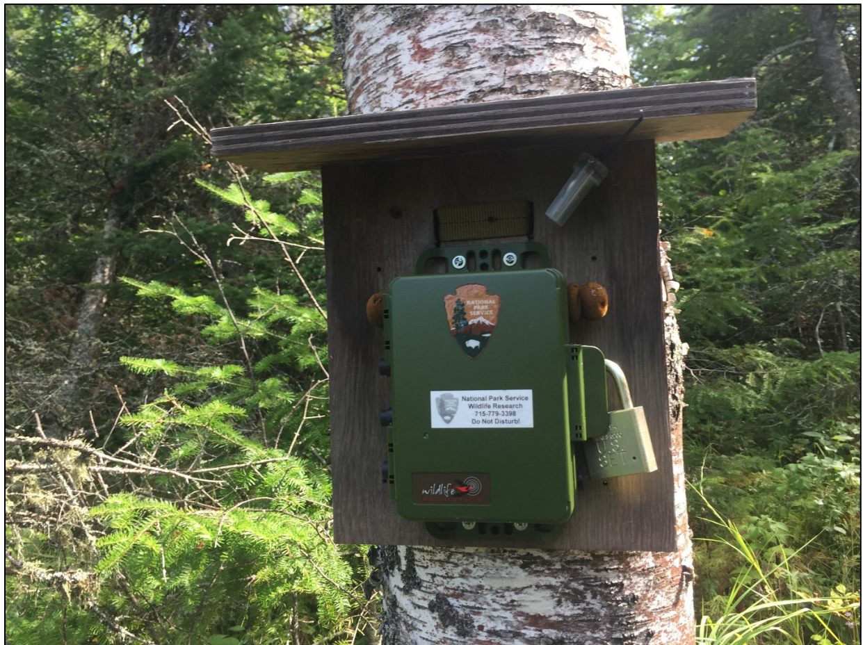
Figure 2. Example of automated recording system (ARS) deployed in the field. This device is attached to a backer board with a strap around the tree. The temperature logger is attached under the roof of the backer board ( upper right ).
