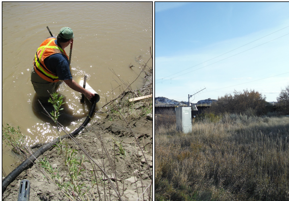
Figure 3. A sonde device is used to measure water quality in the Little Missouri River at Theodore Roosevelt National Park and it is installed within a pipe for protection (left panel). The United States Geological Survey Little Missouri gaging station (06336000) is set up for real-time data transmission via satellite (right panel). Photographs courtesy of USGS, station 06336000.
