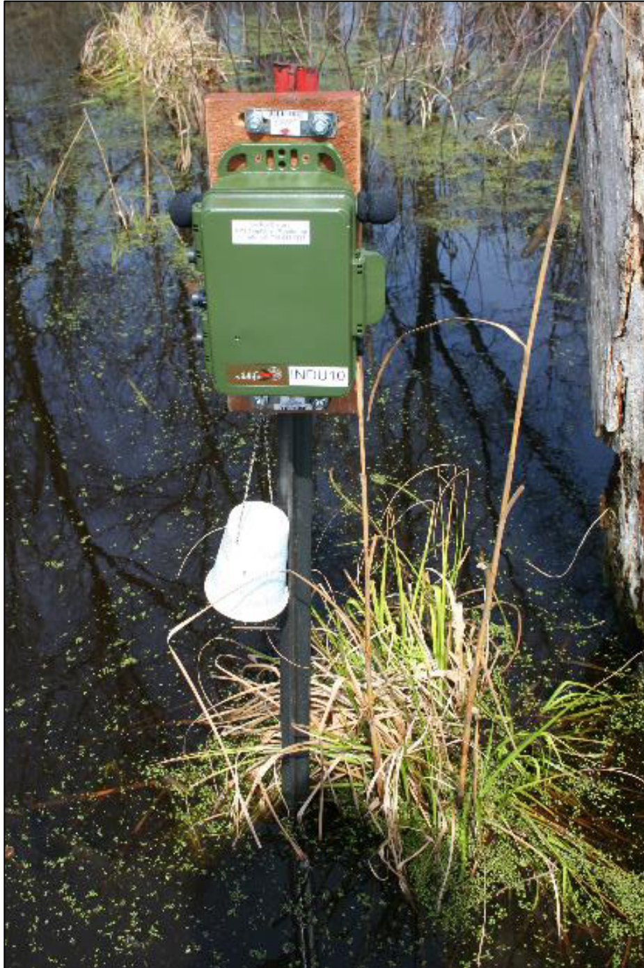
Figure 2. Example of automated recording system (ARS) deployed in the field. This device is attached to a backer board and strapped or bolted to a tree or post. The temperature logger is situated nearby within a solar shield.
