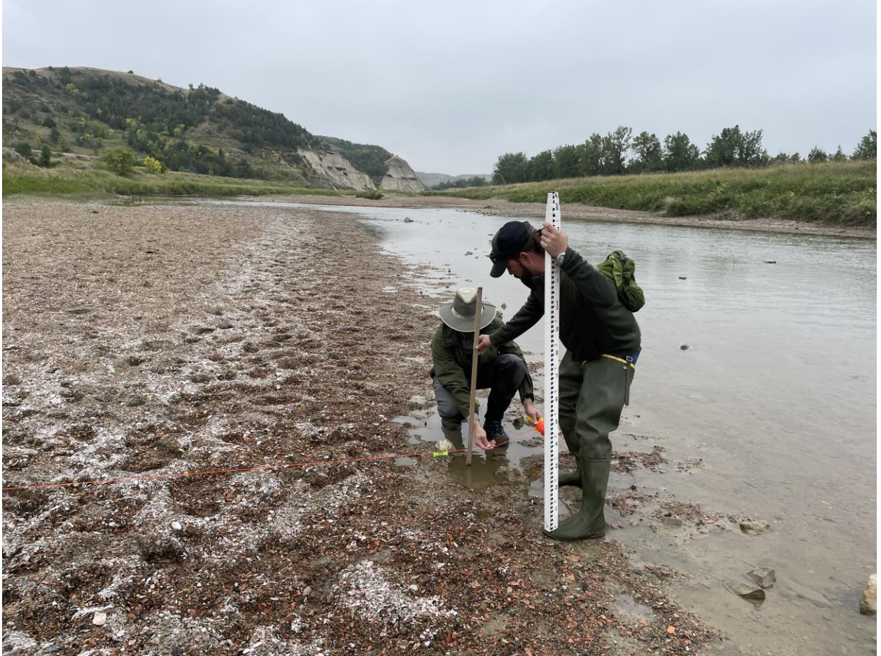
Figure 10. Measuring water depth at base of bank. Chaining pin with line is placed at base of bank. Line is extended to water's edge and held level against a meter stick to determine the negative water depth of the base.
