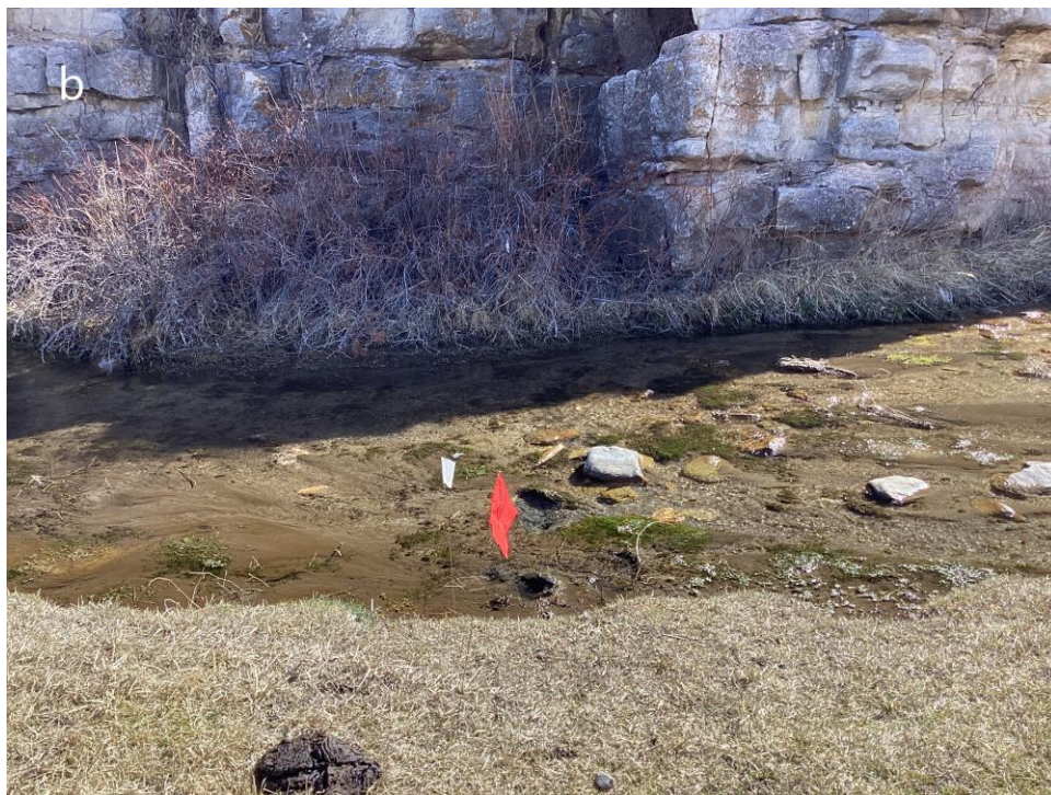
Figure 3b. Left bank photo: Take from right bank, put left bankfull flag in view. Focus on water's edge and bank surface.
