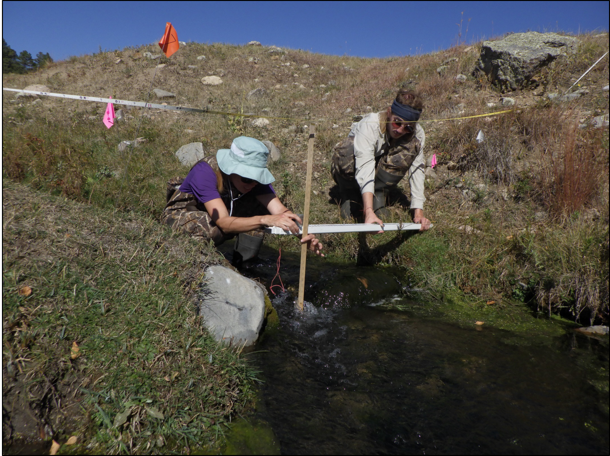
Figure 7. NGPN crew takes bank-full measurements at Transect 7.
