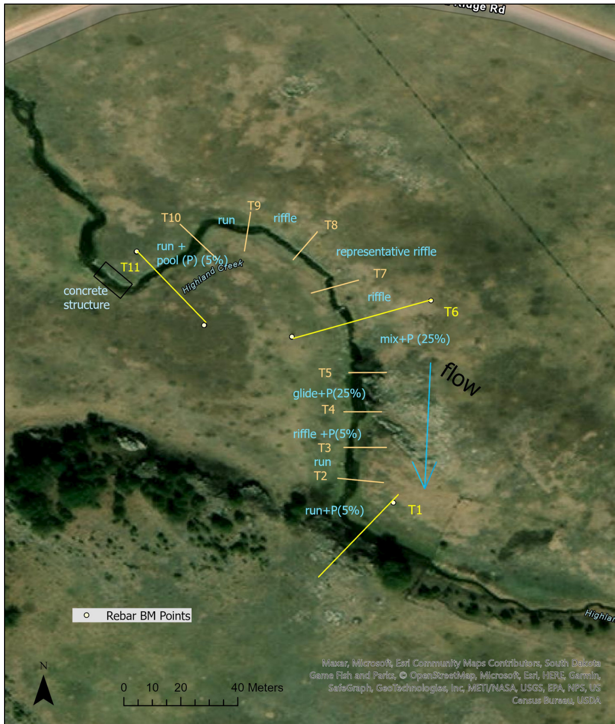
Figure 2. Layout of sampled reach of WICA stream channel monitoring site WICA SCM 001. Transects number 1-11 running from down to upstream. The dominant geomorphic channel unit is noted between each reach.
