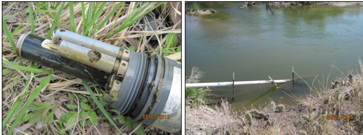
Figure 4. A sonde device is used to measure water quality in the Laramie River at Fort Laramie National Historic Site. The United States Geological Survey Laramie River gaging station (06670500) is set up for real-time data transmission via satellite. Photographs courtesy of NPS.
