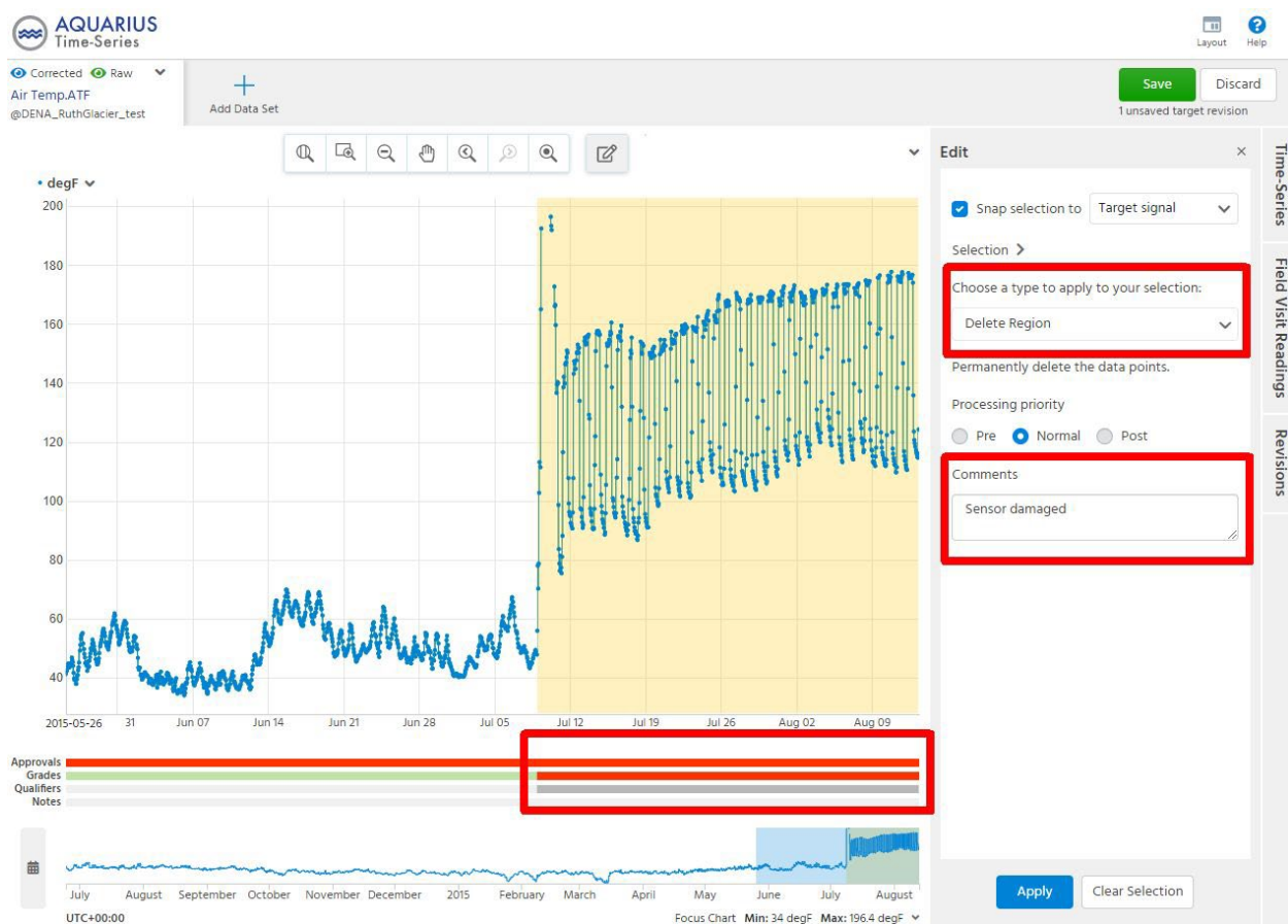
Figure SOP 11-18. An example of data retrieved from a damaged air temperature sensor. Erroneous measurements on June 8. The “Delete Region” correction action deleted all values during the selected time period. A custom comment (“Sensor damaged”) was added to describe the delete region action. For damaged sensors, the quality grade for the time period should also be set to “-2- Unusable” with a descriptive note added to describe the reason for grading.
