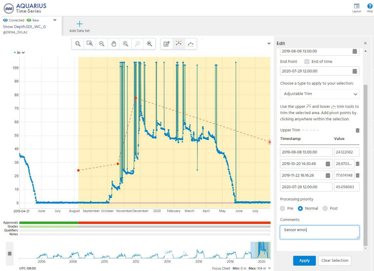
Figure SOP 11-20. Data corrections for a snow depth time series. The adjustable trim edit action suppresses all values above the user-defined pivot points.
