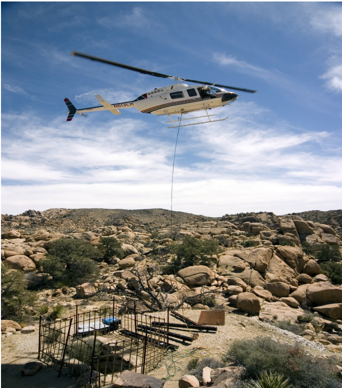
Figure 2. To protect fragile landscapes, heavy equipment and supplies can be airlifted from the closest park roadway. (NPS)
