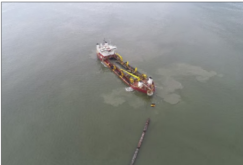
Figure C-2. Hopper-style dredge (COASTAL SCIENCE & ENGINEERING, INC. [CSE]).
