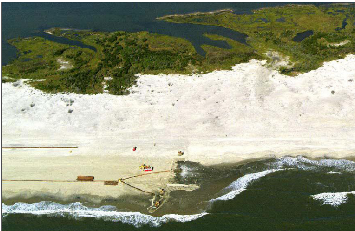
Figure 2. Beach nourishment was implemented at Assateague Island National Seashore, Maryland to mitigate some of the sediment lost from the beach since the construction of the Ocean City Inlet jetties. 2002 photograph (USACE).
