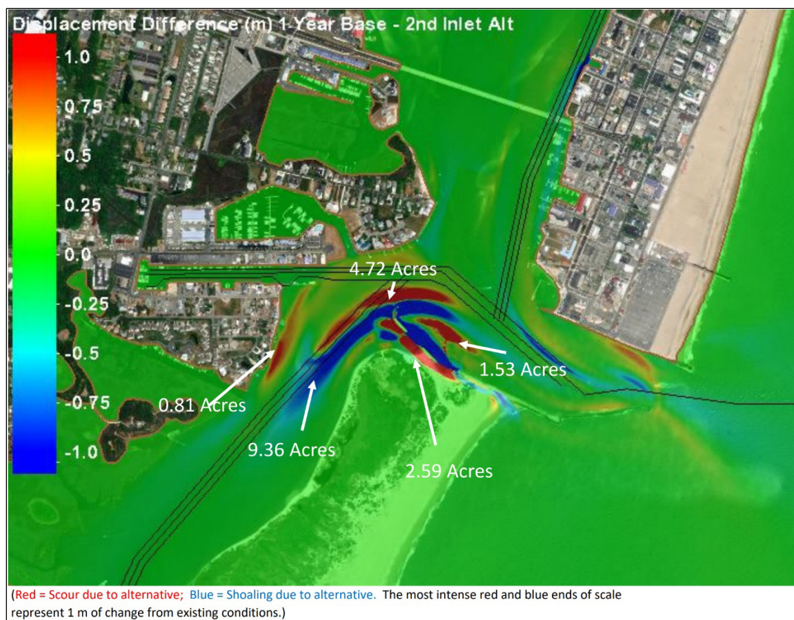
Figure D-4. 2D sediment transport modeling shows shoaling in blue shaded areas and scouring in red shaded areas for the proposed action. 2D modeling aids in determining short-term sediment trends and assessment of various alternatives (USACE 2022: Figure 2.4).
