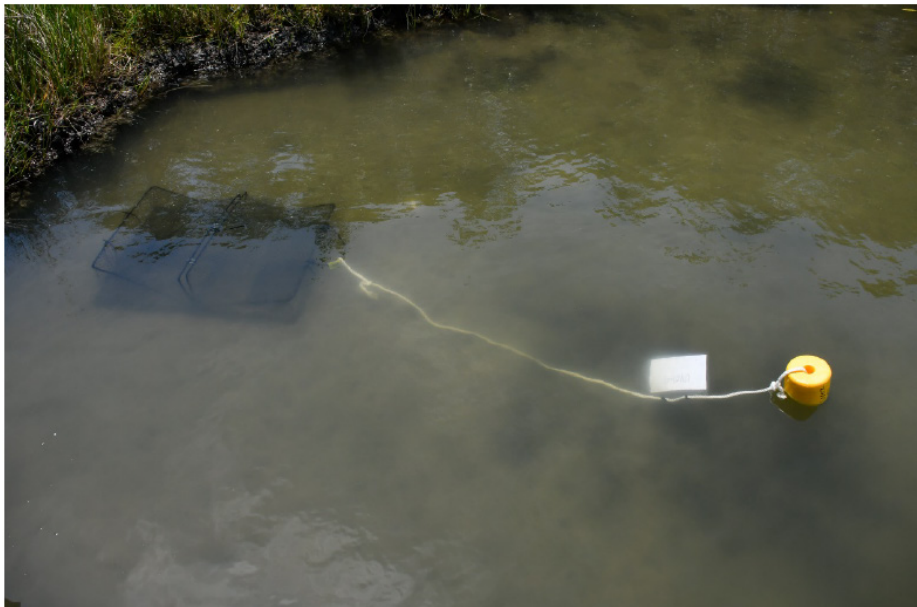
Figure B-2. ID MFB_6030. 2021-07-15. Station UV07-01-PRI. Typical deployment of trap featuring line, buoy, permit information, and station ID.
