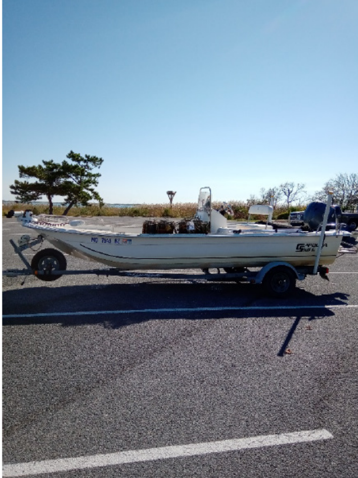
Figure B-3. ID IMG_20210930_100626. 2021-09-30. Assateague State Park. Boat used for field work was a Carolina Skiff. A low draft boat was necessary due to shallow water throughout the study area.
