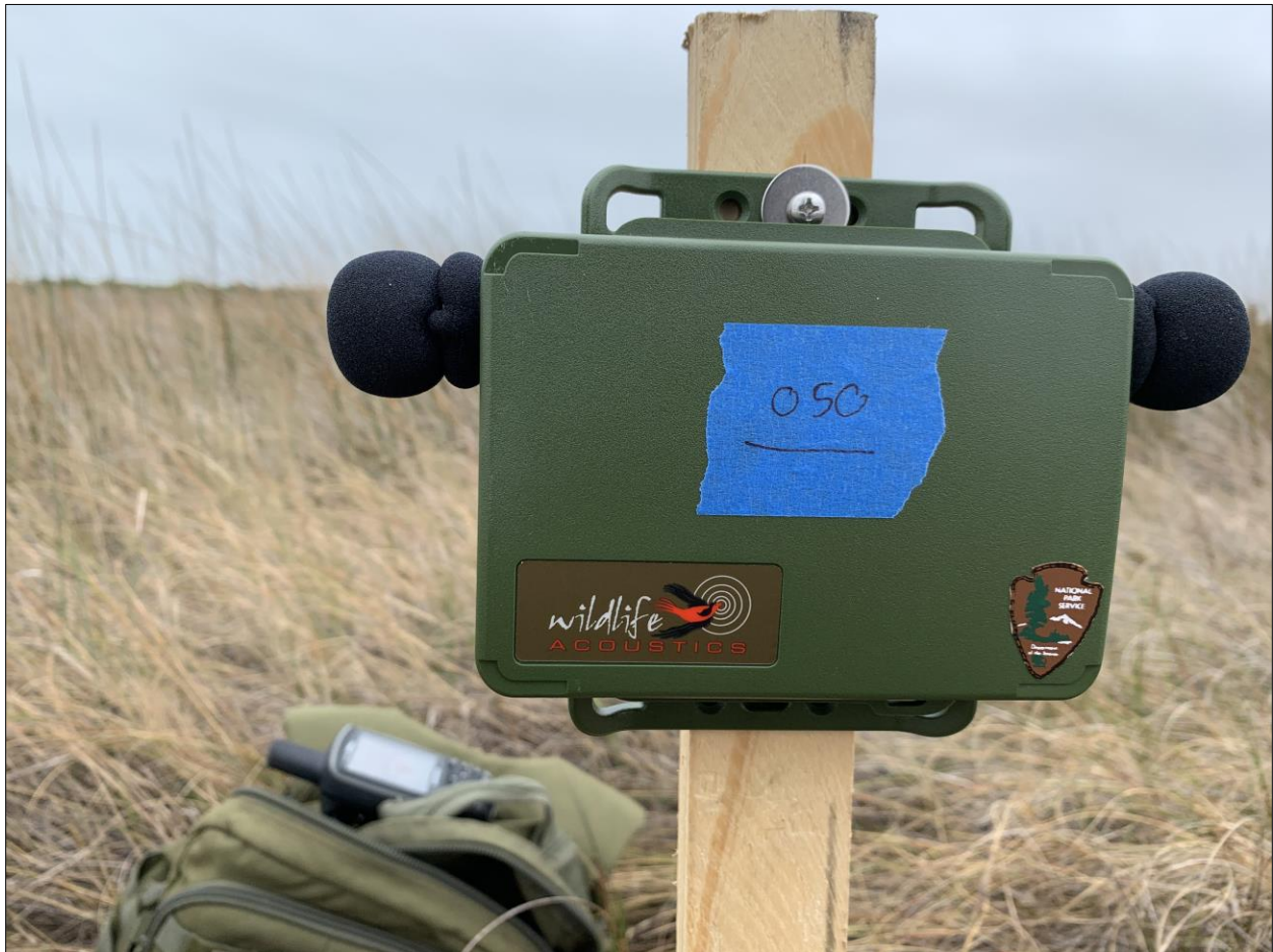
Figure 4. An SM-Mini is mounted on a 4-ft wooden post in the middle of a marsh where no trees are available as mounting locations. Stainless hardware ensures that the wet, salty environment will not overly rust the screw, making later removal easier.
