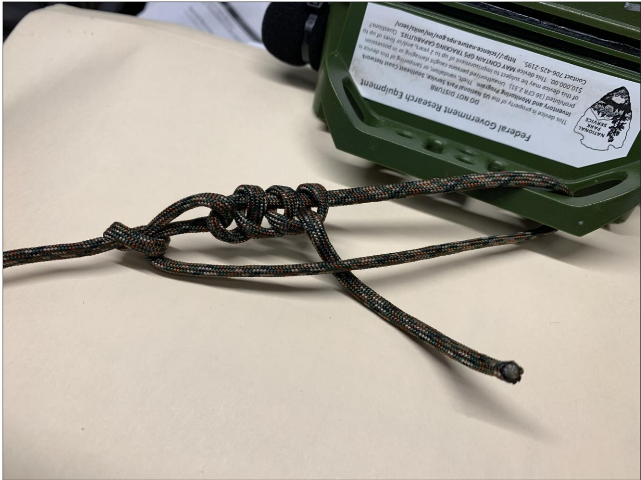
Figure 3. A trucker's hitch is used to cinch down and secure a load. It depends on the far end of the rope being secured first. Create a small loop in the rope before it passes through the ARD bracket. Run the working end through the bracket and back through the small loop in the line. Draw down tight on the working end and secure the line with a few half-hitches while tension is maintained. It is possible to generate a great deal of tension on the rope using this knot. The example knot is tied very loosely for illustrative purposes; in actual use, it is drawn snug.
