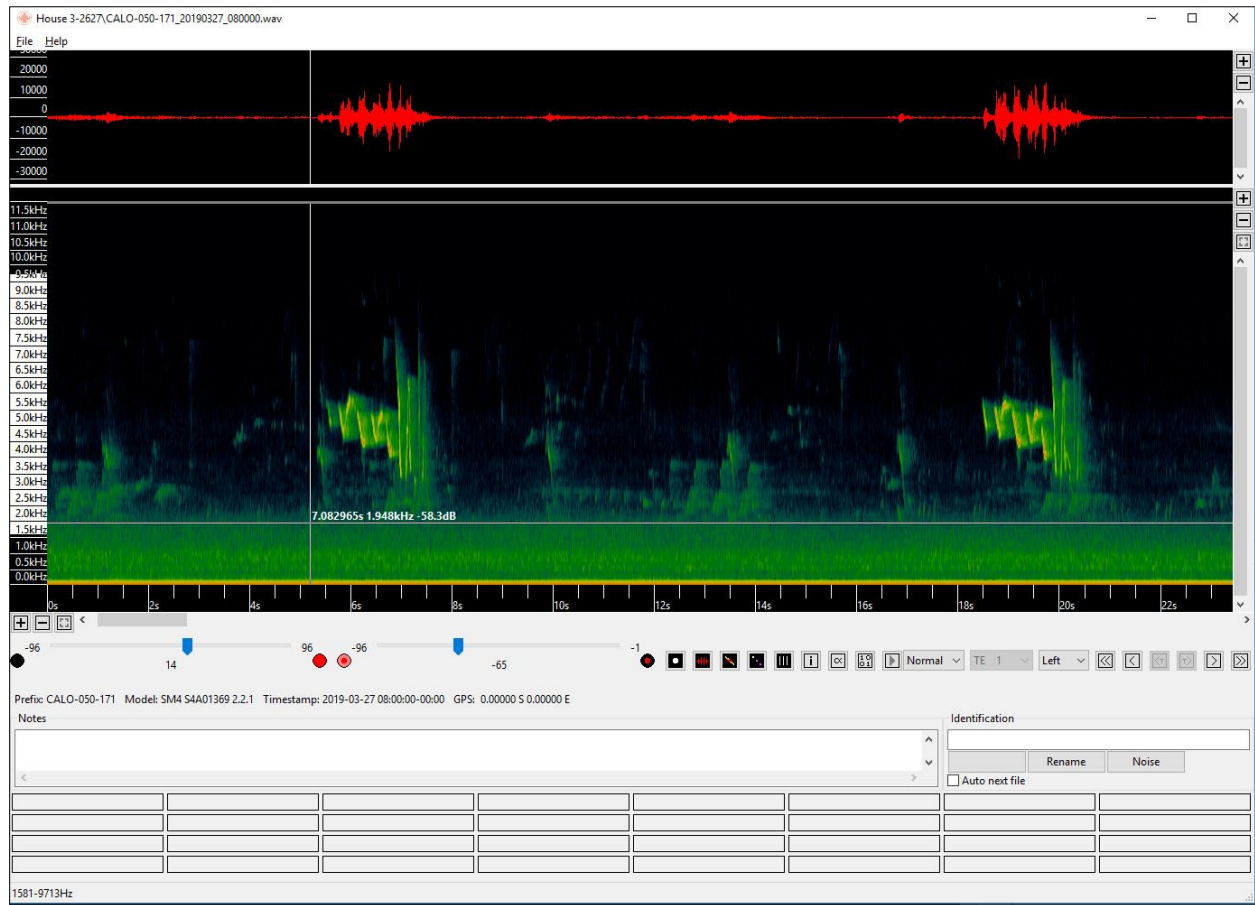
Figure 1. An example screenshot of an audio file being viewed in Kaleidoscope Pro 5. The user has applied a band pass filter (white-highlighted frequency range on the left) to isolate frequencies of interest and minimize background noise. The dB gain was adjusted to play the Louisiana Waterthrush ( Parkesia motacilla ) song clearly, and the mouse is currently indicating the time offset of the first detected vocalization.
