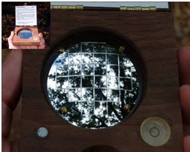
Figure 1. Spherical densiometer grid, users visualize a dot in each corner of the grid ( n=96 dots) and count the number of dots covered by canopy. Note the directions printed on the lid in inset photo.
