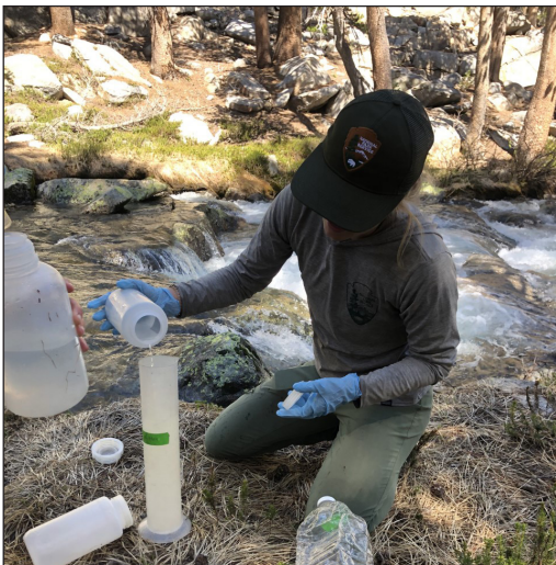
Annalise Decker, Physical Science Technician, prepares for a salt dilution discharge measurement, Lyell Fork Tuolumne River, Yosemite National Park. NPS / R. Hallnan
