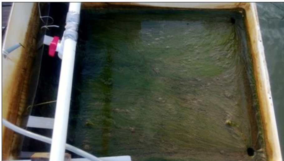
Figure 7.6. A small algal turf scrubber in use at an oyster aquaculture facility for nutrient removal. Algal biomass grows in the trough and locks up nutrients. The biomass is periodically harvested in order to remove nutrients from the system. Photo Credit: Nicholas Ray.
