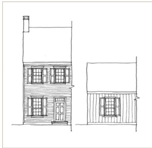
Left: It is common that wood siding for primary buildings is horizontal clapboarding, while outbuildings are more likely to have vertical board siding. Above: Patterns of historic vertical and horizontal siding should be preserved.
