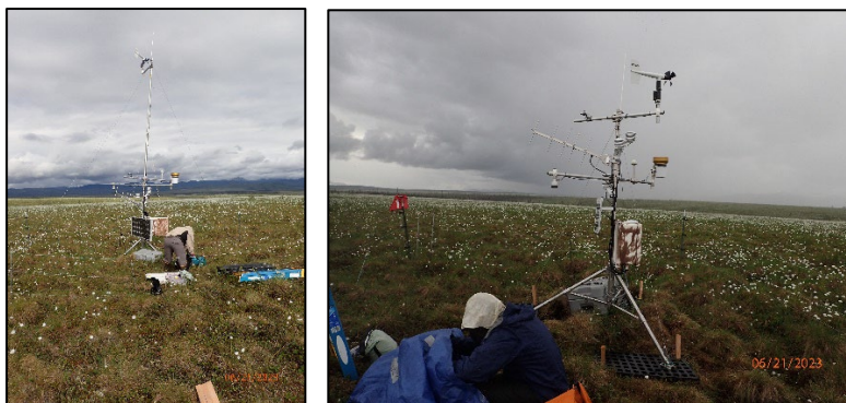
Figure 5. Wigand climate station June 21, 2023 before overhaul (left), and after station overhaul at end of visit (right).
