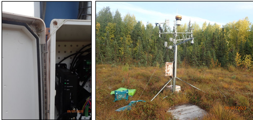
Figure 12. Coal Creek climate station, September 7, 2023. Broken door hinge on enclosure (left). After station visit (right).
