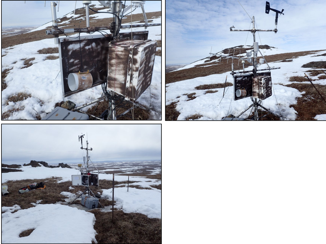
Figure 15. Devil Mountain climate station May 23, 2023. Tipping bucket damage (upper left), more station damage (upper right), station after maintenance visit (lower left).
