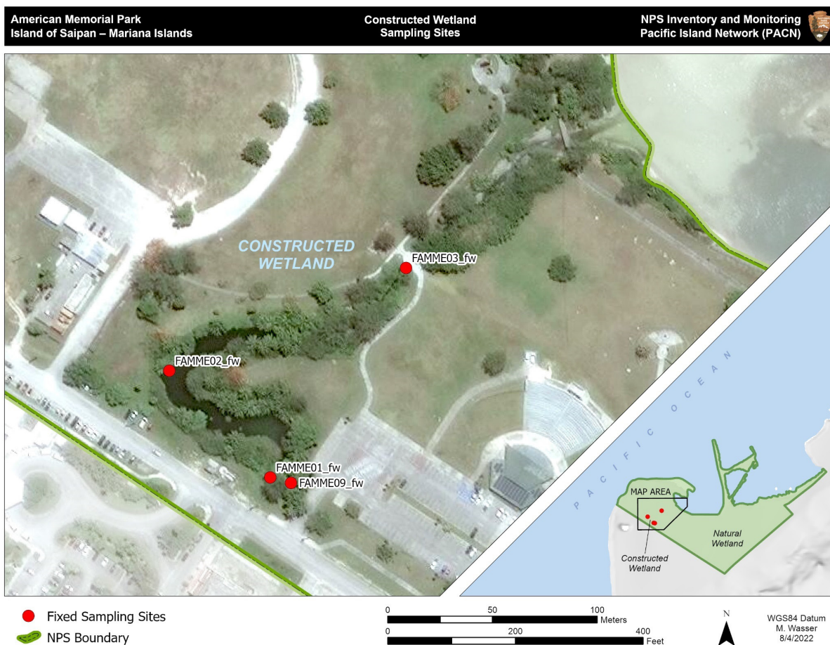
Figure 5. The constructed wetland at American Memorial Park. Sewage-contaminated effluent enters at FAMME01_fw and flows to the shoreline.
