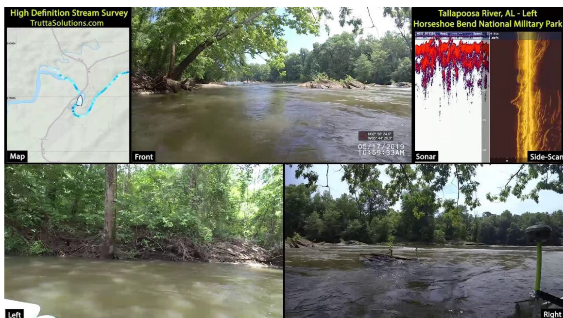
Figure 2: Example of the StreamView Video created for the Tallapoosa River survey near the Horseshoe Bend National Military Park. Boat location can be seen in the map window in the upper left corner. Video Name is in the upper right corner of the video. As noted in the upper right label, this is the StreamView video from the left boat and thus is used for classification of the left bank. The two-boat survey was necessary so that imagery was of sufficient detail along the riverbank to accurate classification. The right riverbank is clearly too far from the cameras for accurate classification.
