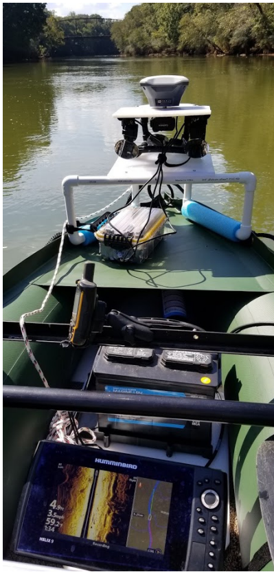
Figure 2: Sonar, Video Camera Array and GPS units used during the Tallapoosa River Survey.
