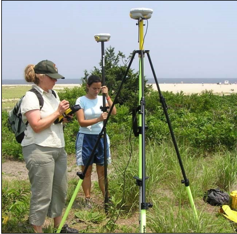
Figure 13. Trimble R8 GPS/GNSS unit (base receiver on tripod, and rover receiver on pole) used for conducting topographical surveys at Gateway National Recreation Area, Sandy Hook Unit.
