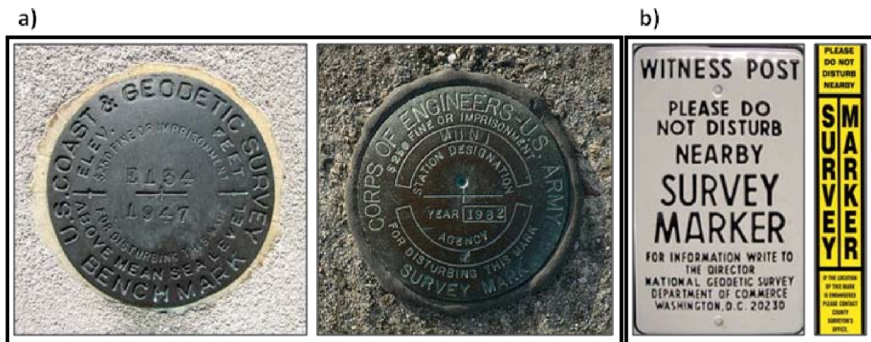
Figure 11. Examples of a) metal disks survey monuments and b) witness post label, established by the US Army Corps of Engineers (USACE) and the National Geodetic Survey (NGS).
