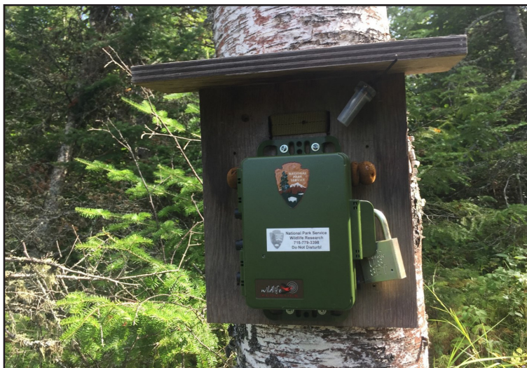
An automated recorder, or “frog logger.” Microphones come out of the top left and right of the box. A temperature logger is attached beneath the “roof” of the backing board. NPS PHOTO
