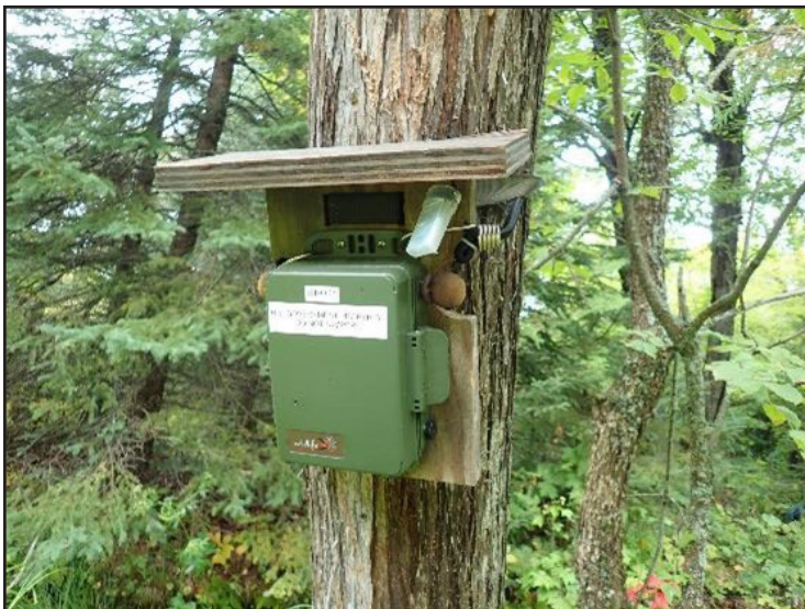
An automated recorder, or “frog logger.” Microphones come out of the top left and right of the box. A temperature logger is attached beneath the “roof” of the backing board. NPS PHOTO
