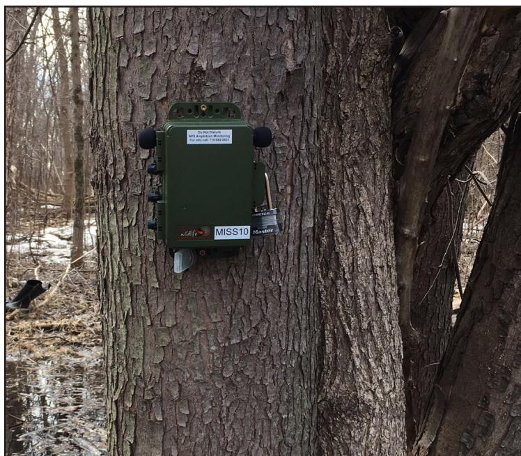
An automated recorder, or “frog logger.” Microphones come out of the top left and right of the box. A temperature logger is attached to the bottom of the unit. NPS PHOTO
