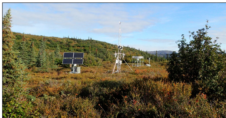
Figure 7. Denali 27N Climate Reference Network Site near the Wonder Lake Campground. The fuel cell and solar panels ( center left) power the site throughout the year.
