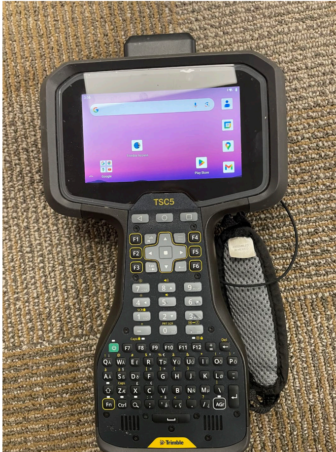
Figure 1: Trimble Access on Data Collector
