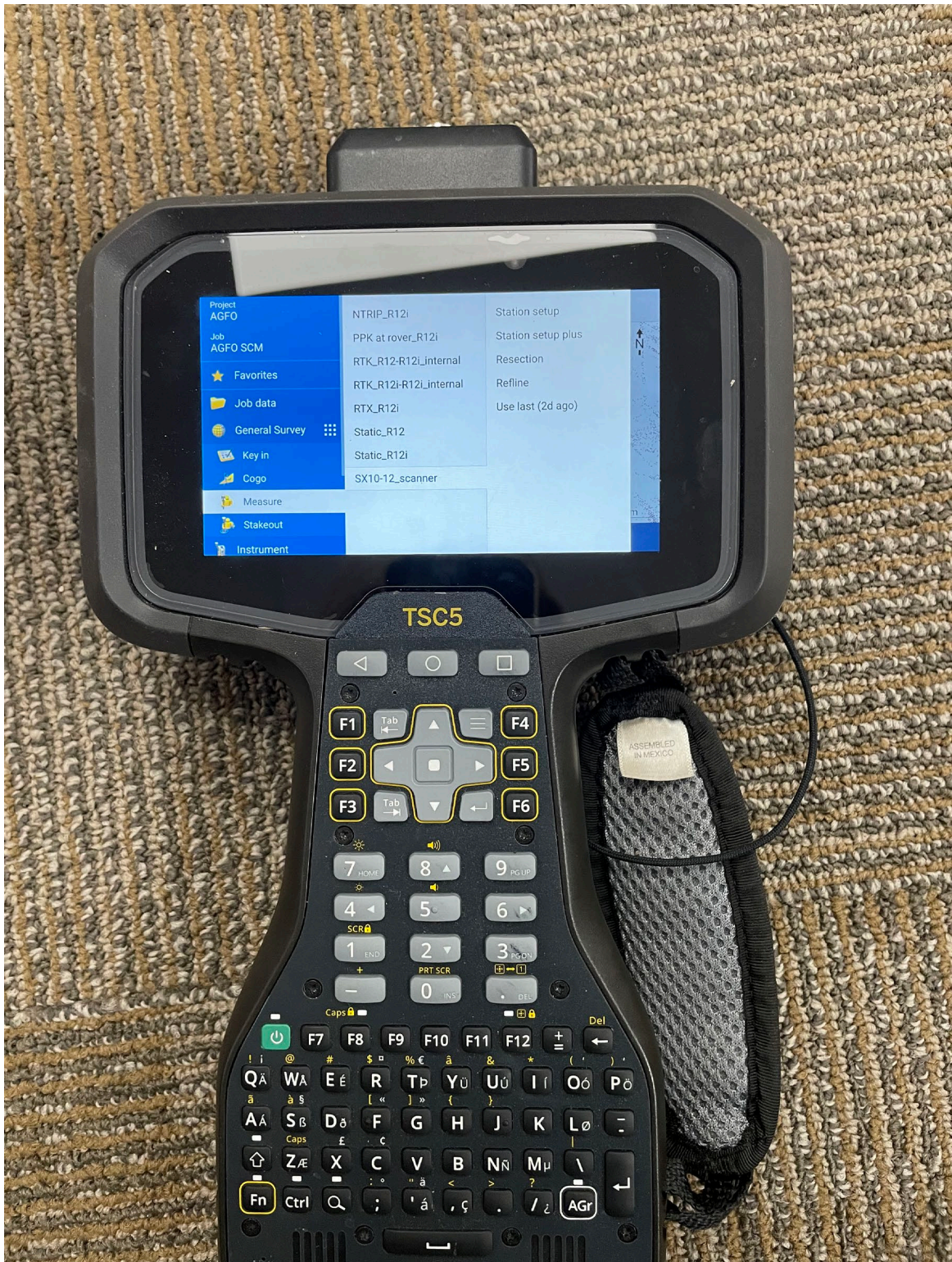
Figure 6. Station setup screen on data collector.
