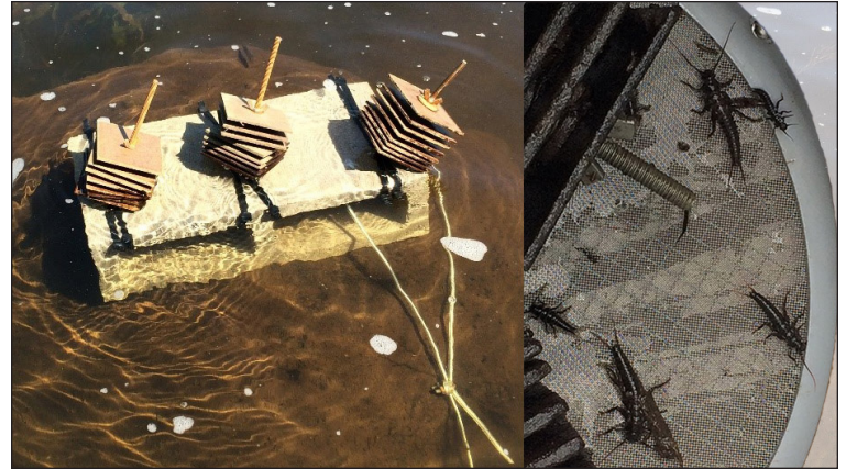
Hester-Dendy macroinvertebrate samplers (left) are a series of wood tiles stacked together on a bolt and placed at least 2 feet below the water surface where there is good streamflow. Aquatic insects colonize the tiles as they would a rock or a log in the river. When removed from the water, the tiles are rinsed to collect insects such as stoneflies (right) that have gathered on them.
