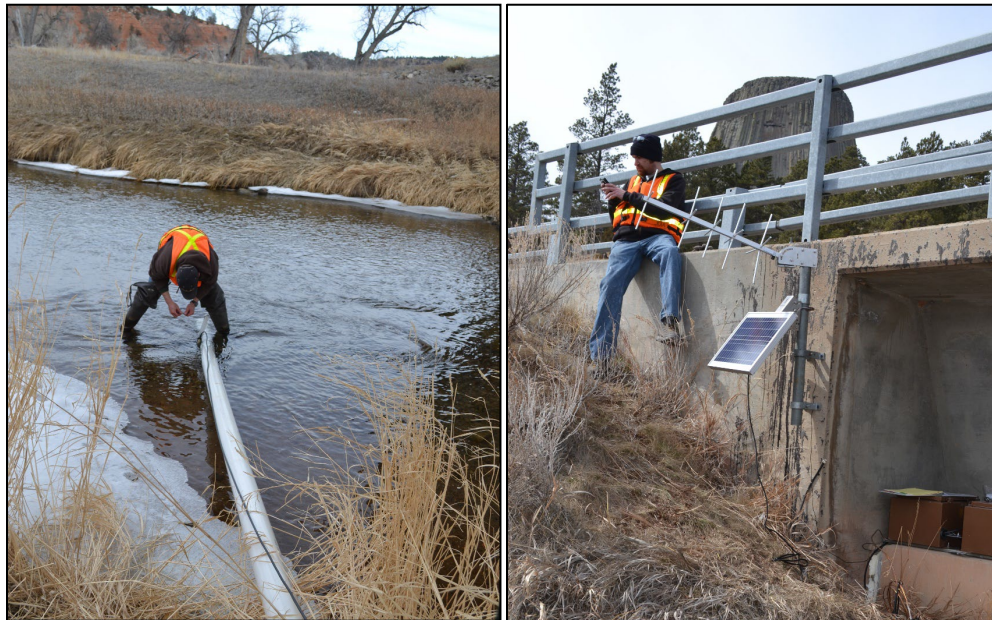
Figure 3. A researcher deploys a sonde device to measure water quality on the Belle Fourche River at Devils Tower, WY. The United States Geological Survey Belle Fourche River gaging station (06427850) is set up for real-time data transmission via satellite. Photographs courtesy of NPS.
