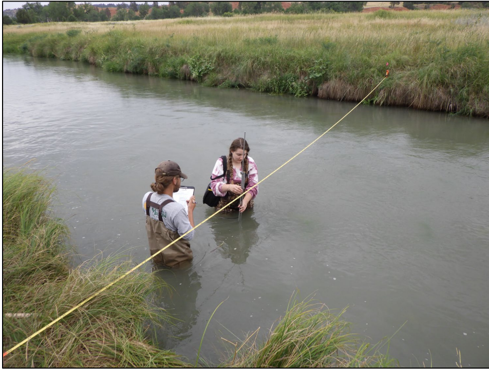
Figure 11. Discharge was measured at the upstream end of the site, along the T11 detailed transect.
