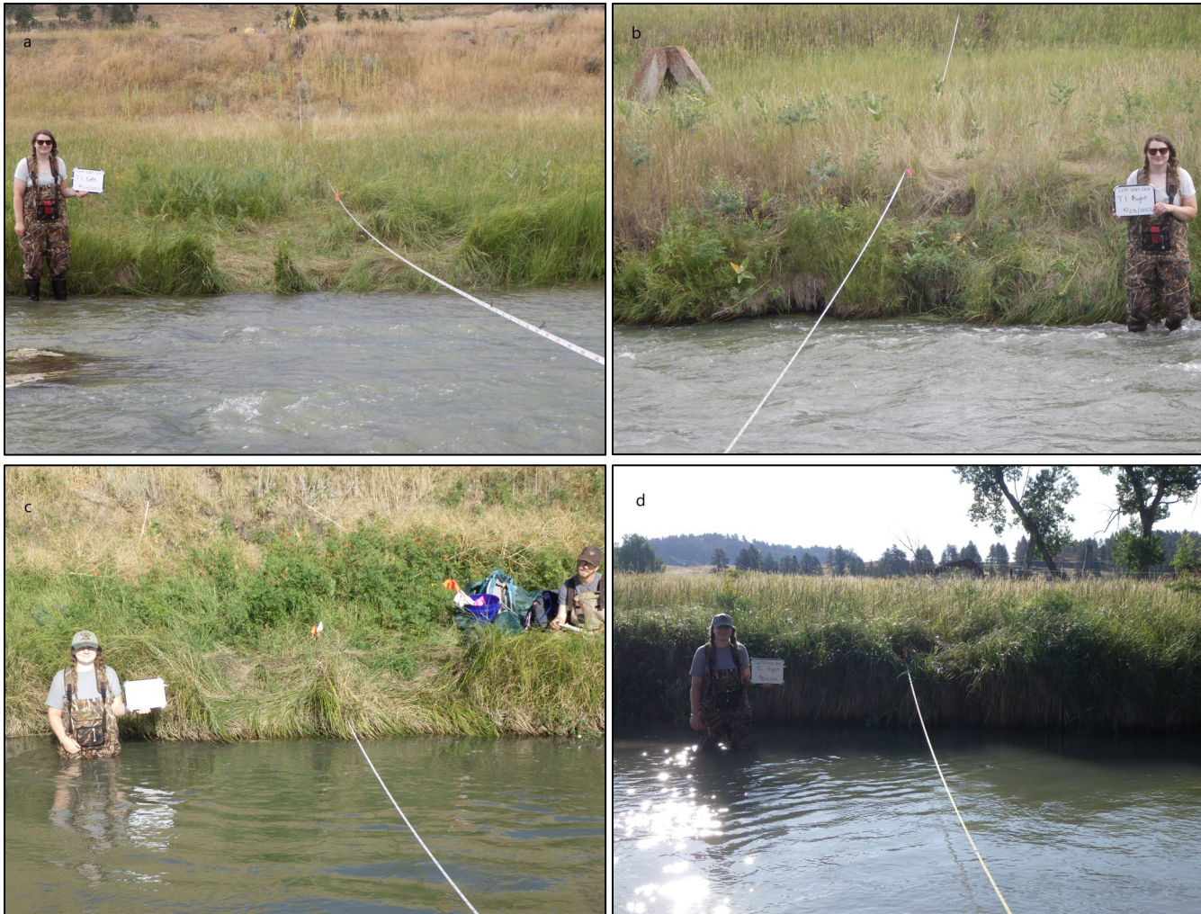
Figure 9. Transect 1 shows little erosion and has bank stability of score of 7.50 on the left bank (a) and 9.50 on the right bank (b). Transect 11 shows high areas of erosion and has bank stability of score of 12.5 on the left bank (c) and 12.5 on the right bank (d). While the right bank at T1 did have a .08 m by .07 undercut, undercutting was much more severe at T11 with a .22m x .42 m undercut on the left bank and a .12 x .1 m undercut on the right bank.
