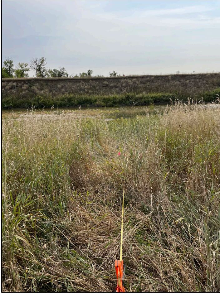
Figure 7. View of detailed transect from the LBM at T6 showing the steep right bank which is located in the middle of the cutbank meander.
