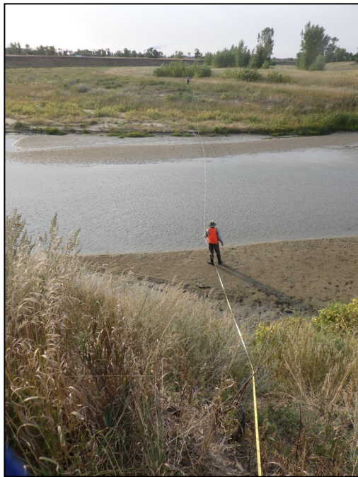
Figure 14. Discharge was measured at the downstream end of the site, along the T1 detailed transect.
