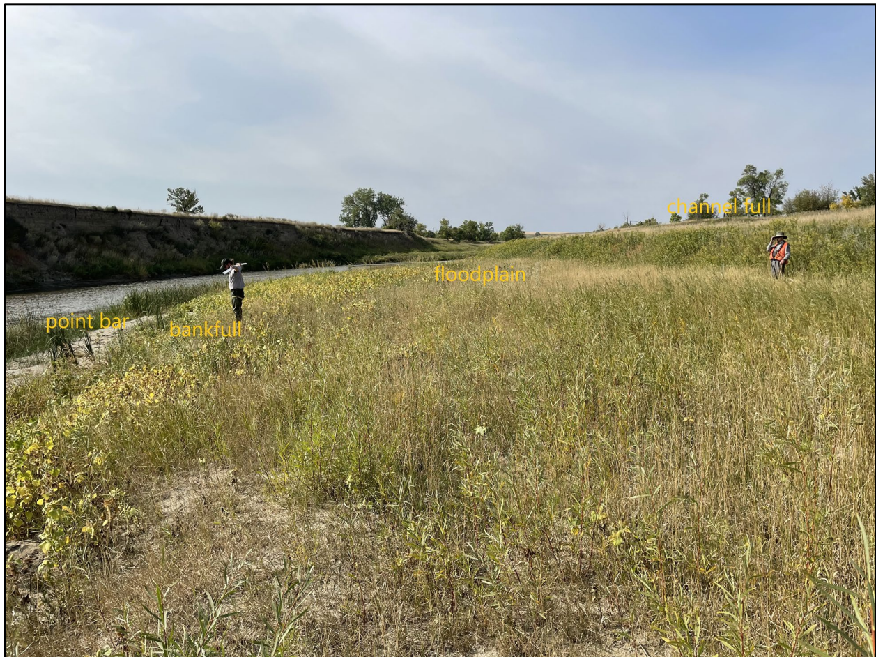
Figure 10. NGPN crew takes bank-full measurements at Transect 5. One crew member stands at bank-full, while the other is at the back of the floodplain.
