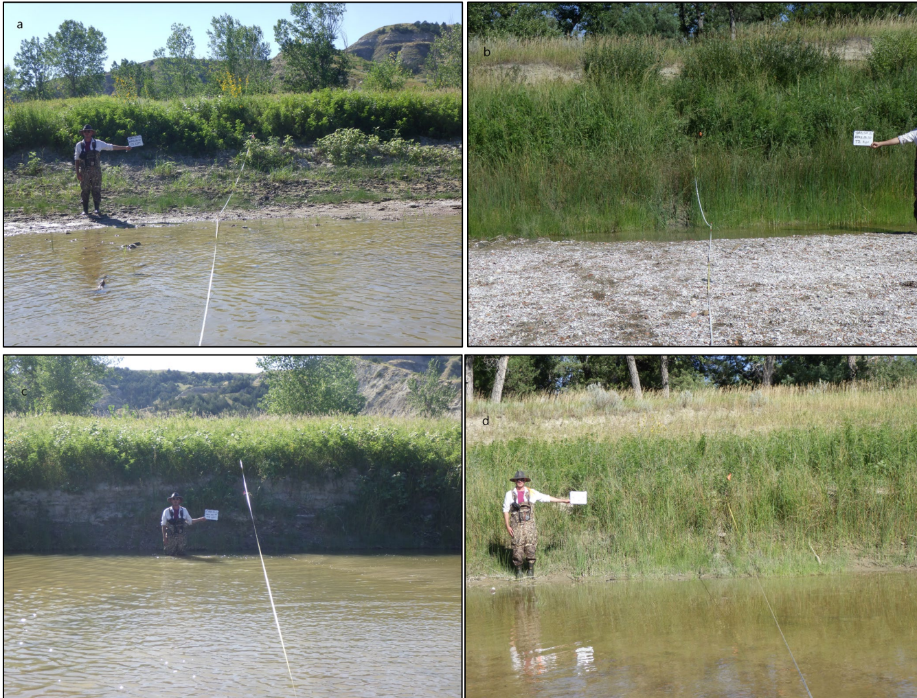
Figure 9. Transect 2 shows little erosion and has bank stability of score of 11.5 on the left bank (a) and 9.50 on the right bank (b) and is considered “at-risk” overall. Transect 3 has a bank stability of score of 17 on the left bank (c) and 13 on the right bank (d) and is considered “unstable”.
