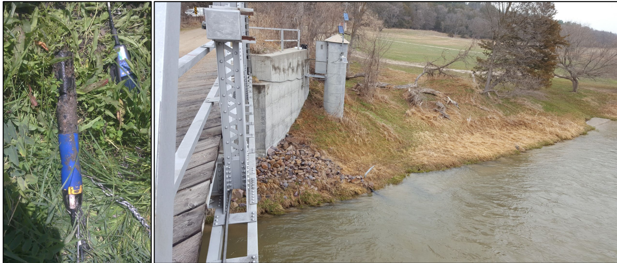
Figure 3. A sonde device is used to measure water quality on the Niobrara River in 2020 at Niobrara National Scenic River (left panel). This sonde is coated in sediment. The United States Geological Survey Niobrara River gaging station (06461500) is set up for real-time data transmission via satellite (right panel). Photographs courtesy of USGS.
