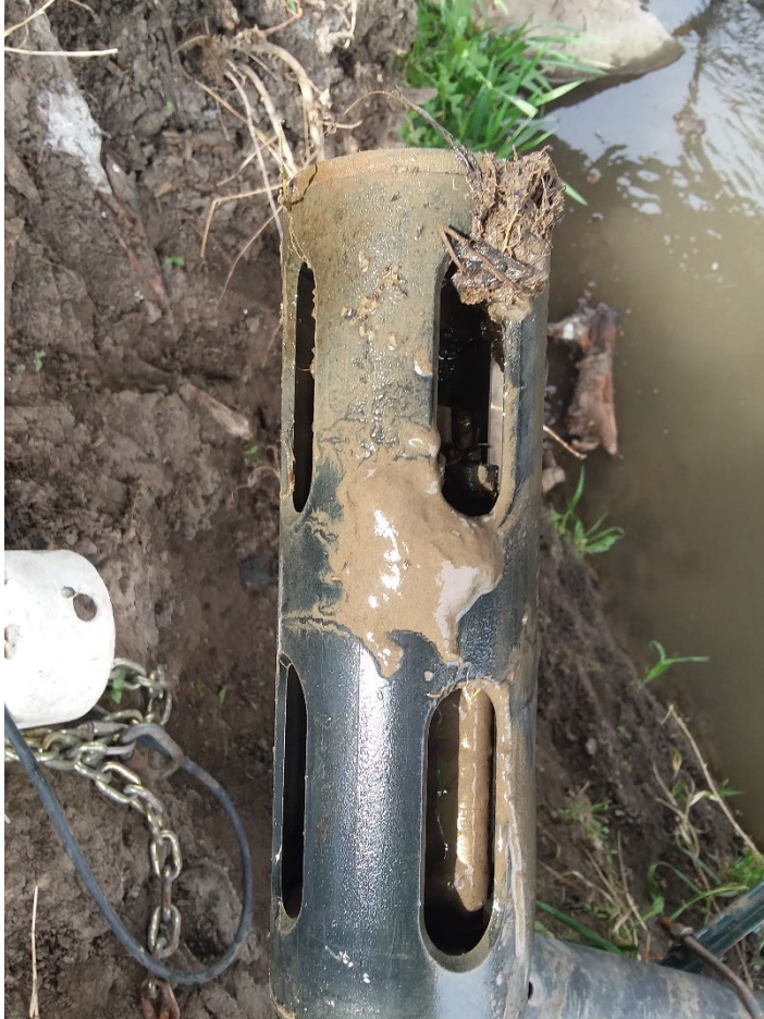
Figure 2. A sonde device is used to measure water quality on Bow Creek in 2021 at Missouri National Recreational River. This sonde is coated with fine sediment.
