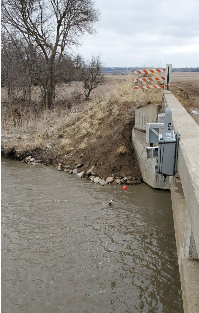
Figure 3. A sonde device is used to measure water quality at 06405500 in a cross-section of the Niobrara River and the radar head for the gage is attached to the bridge.
