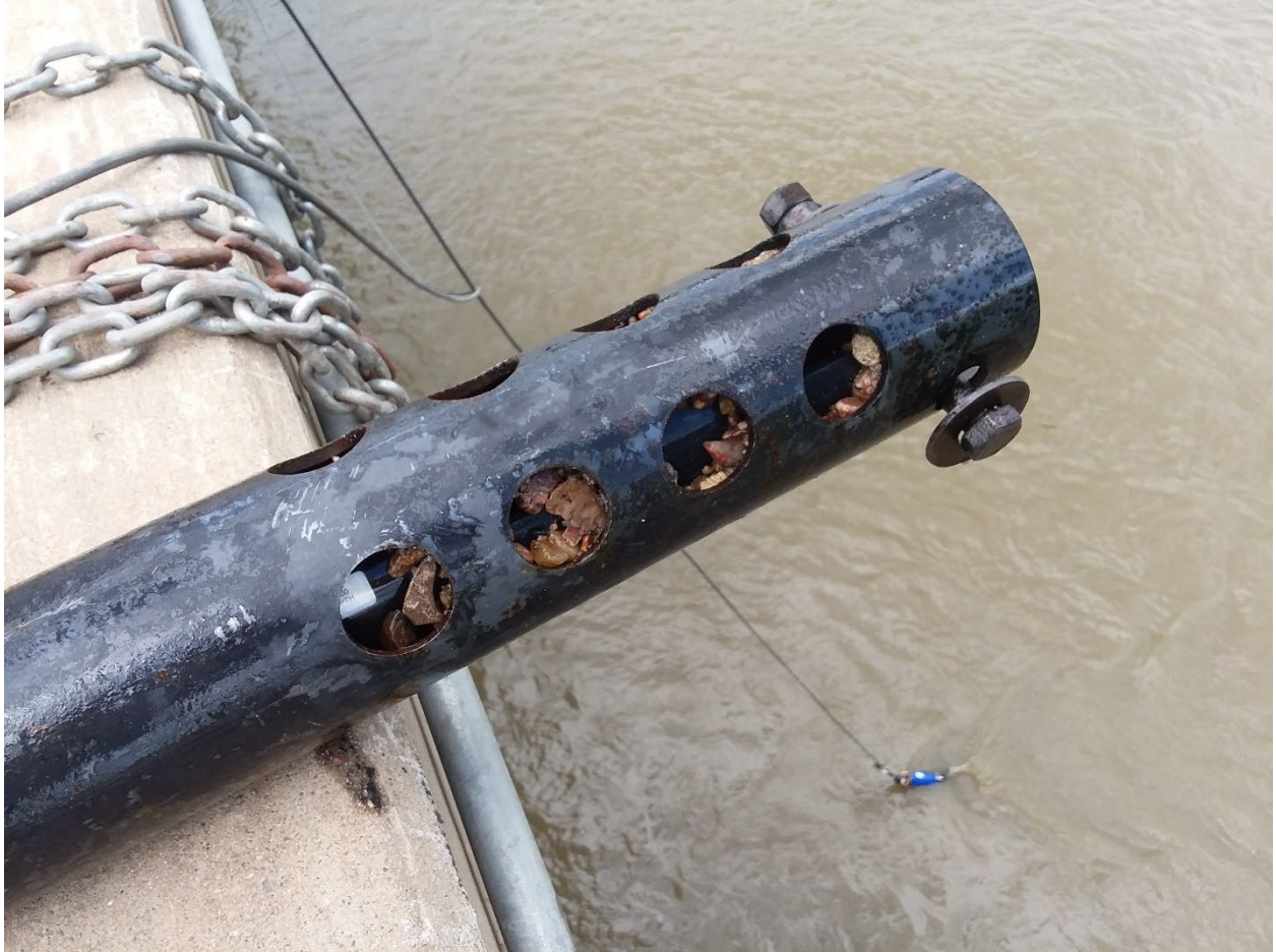
Figure 2. A sonde device is used to measure water quality on the Niobrara River in 2020 at Missouri National Recreational River. This sonde is full of sediment.
