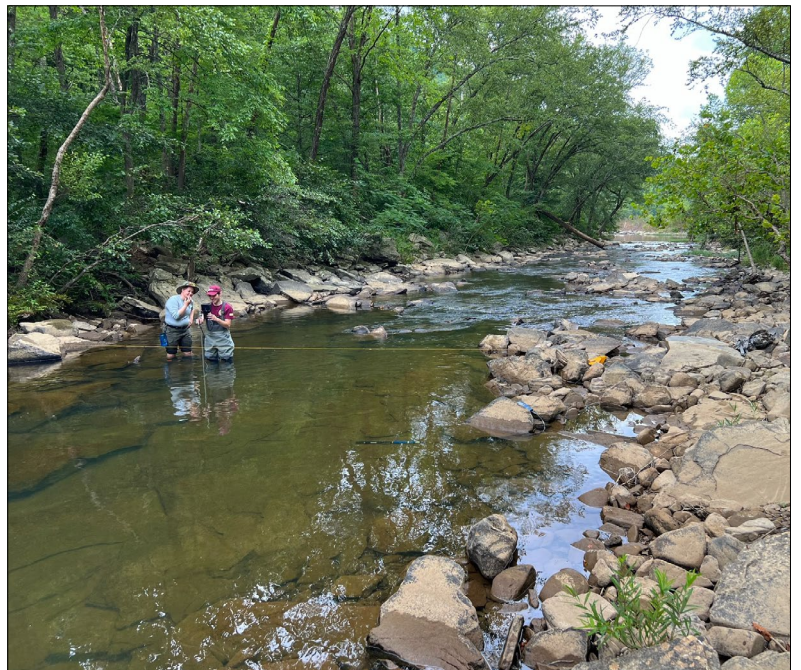
Measuring streamflow on the Emory River upstream of the Obed River confluence. NPS photo / APHN staff.
