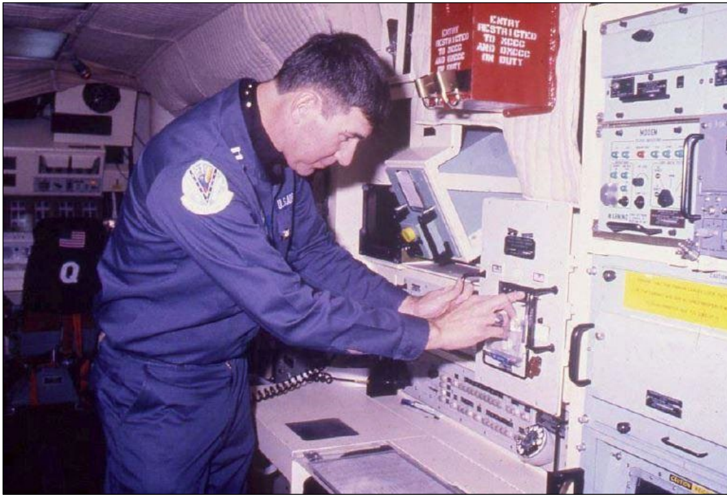
Figure 9. The interior of the launch control center is shown in this ca. 1985 photograph during the Minuteman III period. A missileer is at the deputy commander's communications console. In the distance to the left is the commander's launch control console. Courtesy of Historic Structure Report, Missile Alert Facility Quebec-1 , 2-6.
