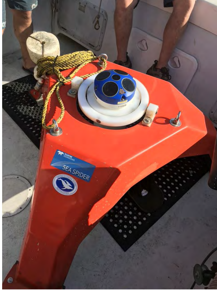
Figure 6. Teledyne RDI Sentinel V20 Acoustic Doppler Current Profiler (ADCP) mounted on a Teledyne Sea Spider seafloor platform.
