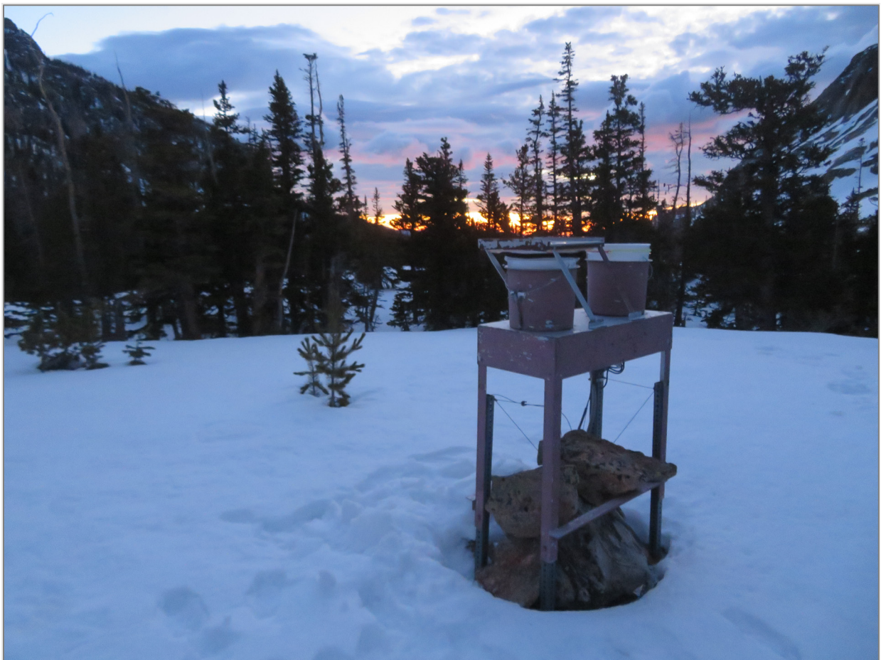
NADP Precipitation Collector at Loch Vale in RMNP (© LISA FOSTER KOSTADINOV).
