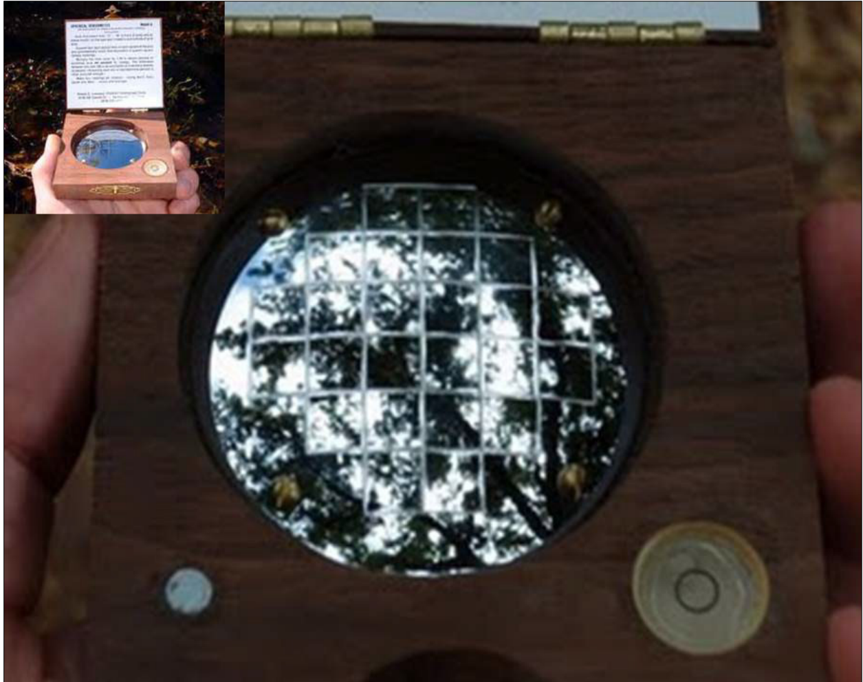
Figure 8. A spherical densiometer grid, illustrating how users visualize a dot in each corner of a grid ( n=96 dots) and count the number of dots covered by canopy. Note the directions printed on the lid in the inset photo.
